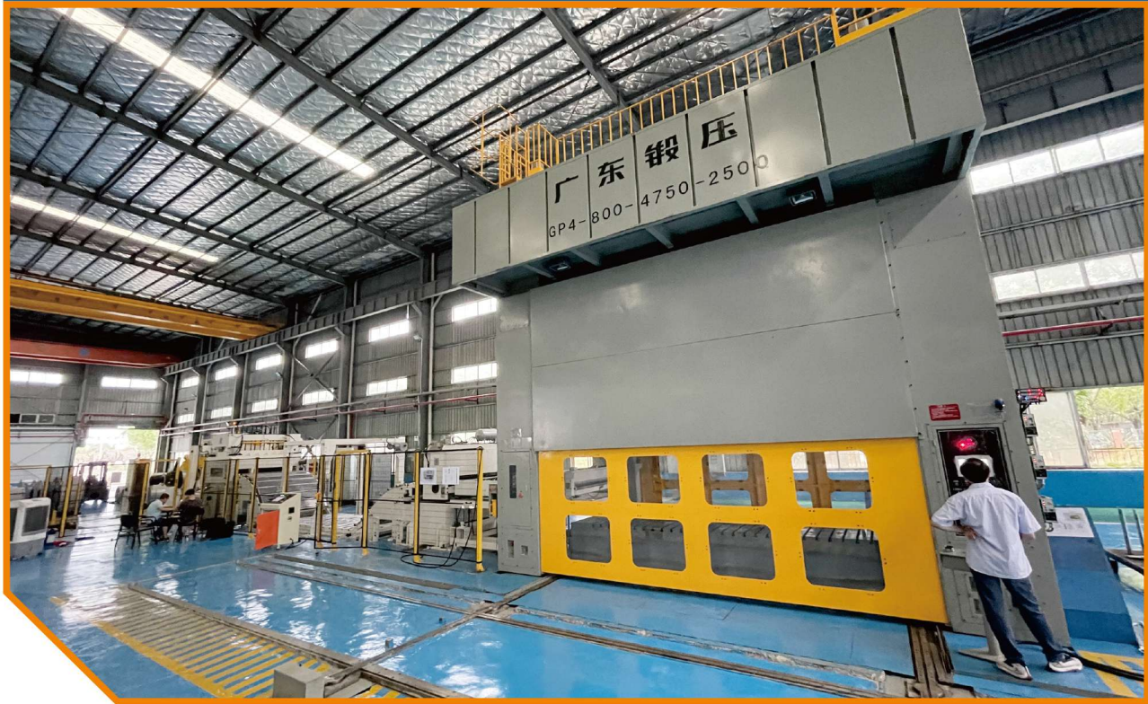
Auto parts industry G2L-600 two-point multi-link press with 3D automatic feeding line
