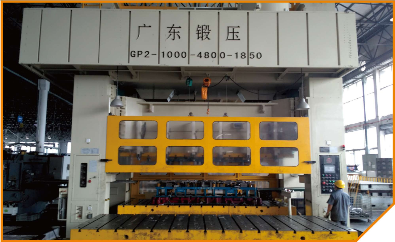
Auto parts industry GP2-1000 two-point press with 3D automatic feeding line
